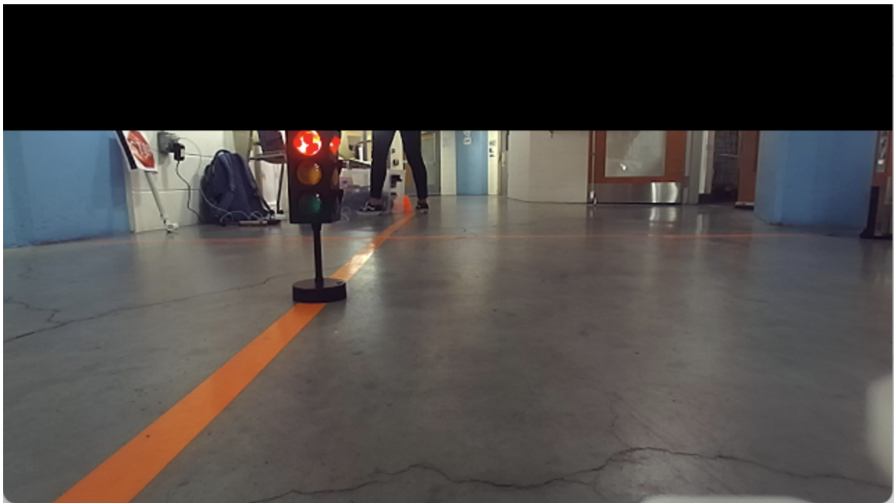
Fig. 12. Case when a green the robot correctly identifies a green light. The green circles are where green contours have been detected in the image and the red circles are where there are red contours. As seen there are green contours on the green light and there are some red contours in other locations of the image.
