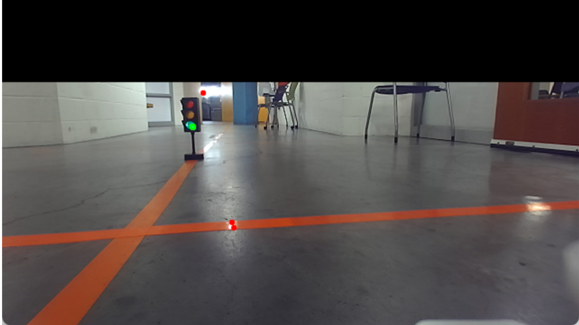
Fig. 12. Case when a green the robot correctly identifies a green light. The green circles are where green contours have been detected in the image and the red circles are where there are red contours. As seen there are green contours on the green light and there are some red contours in other locations of the image.
