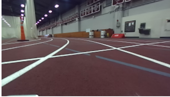
Fig. 1. Example source image frame from the camera. The track the robot is currently on can be correctly identified by the white lines to the left and right of its vision. However, the robot itself may have difficulties with other lanes, intersecting lines, and gray lines, therefore our filtering must account for all these cases.
